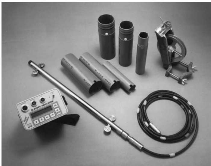
FIG. 1 Typical Components of Inclinometer System
